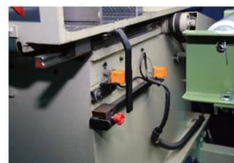
前後近接開關 Front and rear proximity switch
