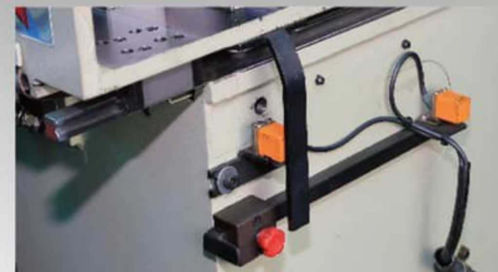
線軌加強工作檯面穩定 Line rail increases work platform stability
