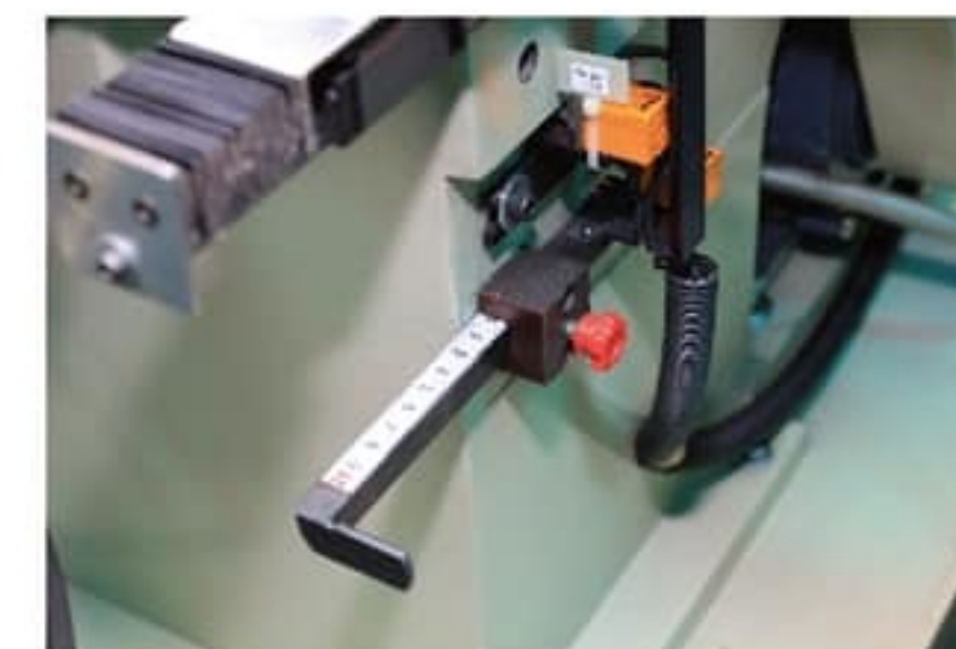
前後近接開關 Front and rear proximity switch
